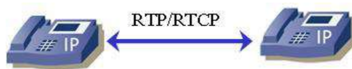
Figure 6.10 - The IP Phone to IP Phone Functional Area
